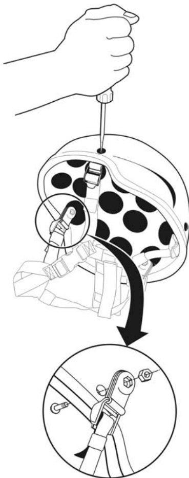
Figure 1. Hardware Installation (MSA TC2000).
